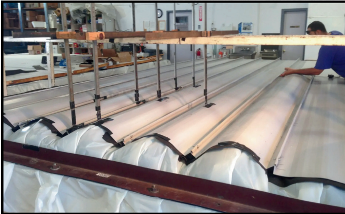
ASTM E 1592 test with pressure being applied
