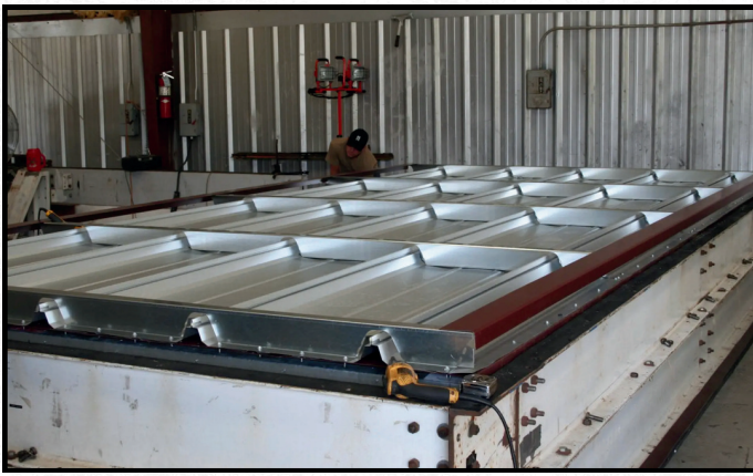
Prior to new panel installation for ASTM E1592 testing
