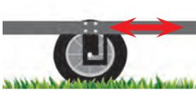
Engage wheels to move tool around, disengage to start working.
