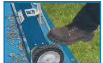
Magnet's quick release action, may be operated by foot or hand.
