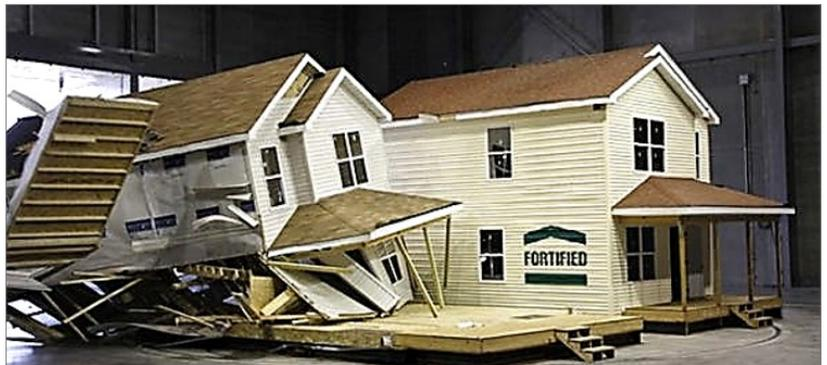
Engineers at the Insurance Institute for Business & Home Safety research center can blast homes with tornado-strength winds generated by 105 giant fans. Drop in a half-million gallons of water or ice from the ceiling, and they can simulate hurricanes and hailstorms.
