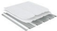
**GAF Acrylic Coatings** provide protection against normal weathering, aging, and UV exposure on roofs that need moderate restoration and extension of life. They can be used on BUR, SBS, APP, metal, structural concrete, aged single-ply, SPF, and previously coated acrylic roofs. Acrylic Top Coat and High Tensile Acrylic Top Coat meet ASTM D6083, are CRRC Rated (white only), FM Approved\*, Classified by UL in accordance with ANSI/UL 790†, and Miami-Dade County Product Control Approved.
