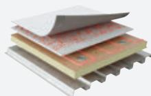
Apply adhesive in a spatter pattern, apply the membrane, weld the seams and smooth with a weighted roller. This membrane installation method is up to 50% faster than installation of smooth membrane with traditional solvent-based bonding adhesive, increasing productivity, requires no expensive equipment, and the fleece backing offers additional puncture resistance.<sup>1</sup> Qualifies for up to a 35-year guarantee\*. Ideal for most environments.
