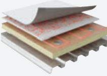
Apply adhesive in a spatter pattern, apply the membrane, weld the seams and smooth with a weighted roller. This membrane installation method is up to 50% faster than installation of smooth membrane with traditional solvent-based bonding adhesive, increasing productivity; requires no expensive equipment; and the fleece backing offers additional puncture resistance.† Qualifies for a 30-year guarantee.\*
