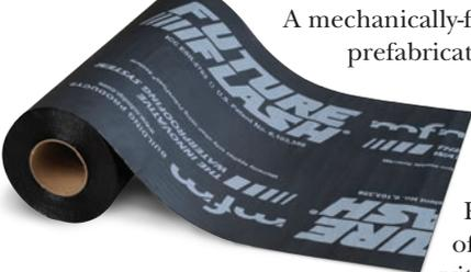
A mechanically-fastened, 25 or 40 mil prefabricated waterproofing membrane that is designed for use around windows and doors, under stucco and other exterior wall systems. FutureFlash® is constructed of two high-performance films with a core of specially formulated rubberized asphalt sandwiched between them. The outer polyethylene film is extremely tough and resistant to tear.
