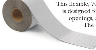
This flexible, 70 mil waterproofing tape is designed for curved window and door openings, as well as sill pan flashing. The self-sealing membrane consists of a rubberized asphalt adhesive laminated to a cross-laminated polyethylene crepe film that allows the product to stretch to curved shapes. Available only in individually wrapped rolls.
