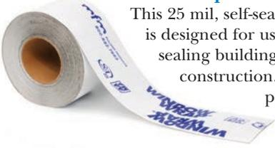
This 25 mil, self-sealing waterproofing tape is designed for use around windows and doors, sealing building seams and general construction. It is composed of a white polymer film and aggressively bonds to the substrate and window flange to prevent damage from water penetration. Available only in individually wrapped rolls.
