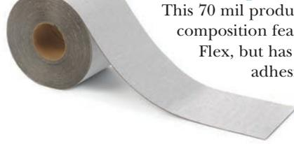
This 70 mil product features all the composition features of WindowWrap® Flex, but has a patented PowerBond® adhesive system that aggressively adheres in temperatures as low as 25°F. Ideal for all curved surfaces, this tough membrane is available only in individually wrapped rolls.
