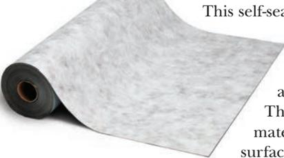
This self-sealing, 30 mil waterproofing membrane is composed of a polyester fabric laminated to a rubberized asphalt adhesive system. The fabric strengthens the material while providing a surface which bonds with most coatings. It is designed to be used around windows and doors, and for taping panel seams and other openings.
