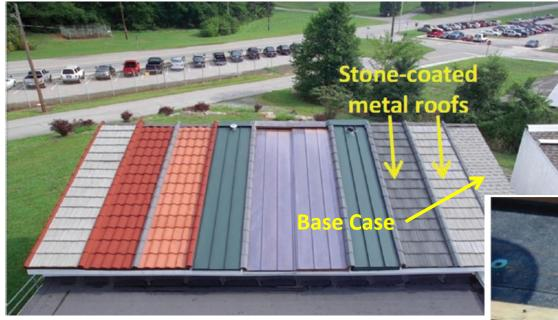
"A painted metal roof on a 4:12 roof slope with a ¾" ASV cavity needed only a 0.1 SR to have the same annual cooling load as a 0.25 SR direct-to-deck metal roof"
