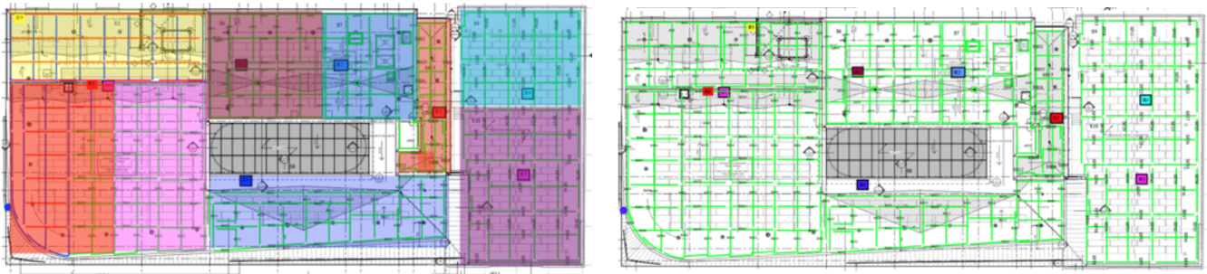
Roof Deck divided into zones for FutureCast Active Install (Left) FutureCast sensor grid gives wide coverage of roof deck (Right)
