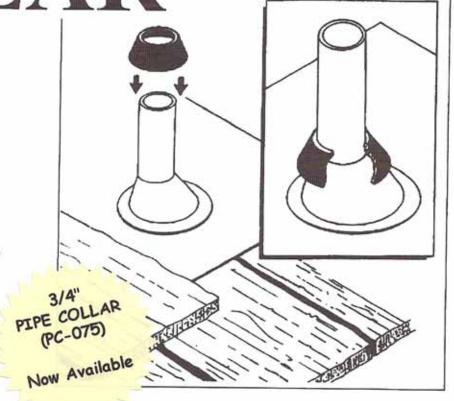
The PIPE COLLAR by Wil-Mar Products was developed to eliminate the problem that exists when sealing a vent pipe to a roof flashing. The PIPE COLLAR is made from a special EPDM rubber compound that meets ASTM D-2000 Standards for hi-lo temperature, oil, ozone and sunlight resistance. It is warranted to last as long as any of the roofing systems being offered today. The PIPE COLLAR's unique
