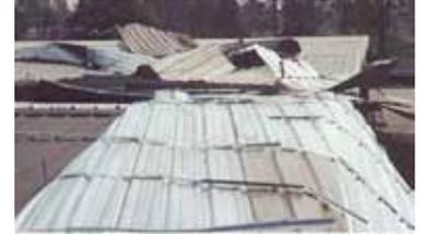
Test showing typical "hat" section failure.
