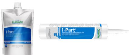
1-Part is a pourable, self-leveling, 100% solids polyether sealant that requires no mixing. It cures with atmospheric moisture to a flexible rubber mass that will not shrink. Available in 10.1 oz. and 28 oz. cartridges or 1/2 gallon pouches.
