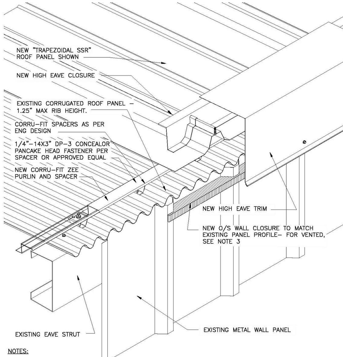
1. ATTACHMENT FASTENERS BY ROOF HUGGER UNLESS NOTED OTHERWISE.
