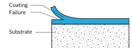
**SUBSTRATE FAILURE (fig 4)**
