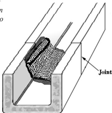
*Metal gutters hanging from eaves need extra protection at seams and fasteners.*
