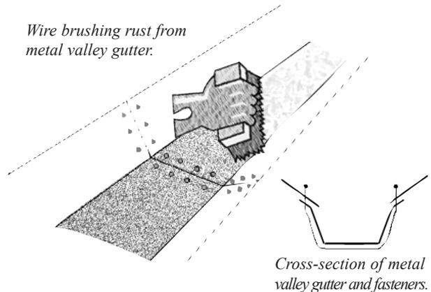
*Cross-section of metal valley gutter and fasteners.*
