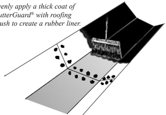
*Concrete gutters require PolyCore™ embedded in GutterGuard® at joints to add reinforcement.*
