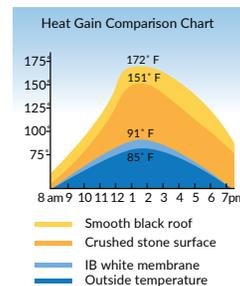
A white IB Roof Systems membrane can reduce your energy consumption and your rising electric bills, by reflecting up to 90% of the heat that normally enters a home through the roof. An IB Roof Systems roof will lower your home's heat gain, and possibly pay for itself.
