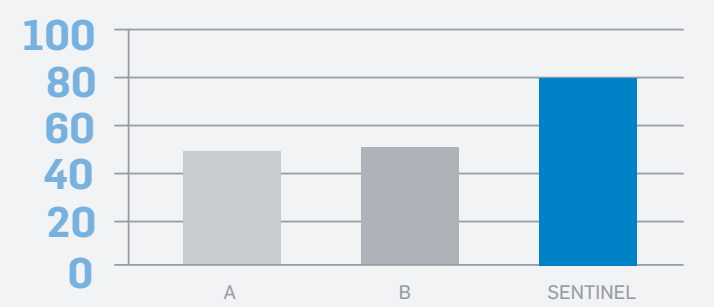
TEAR RESISTANCE - 45 lbf, minimum per ASTM D4434
